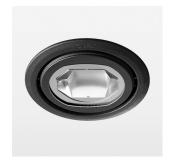
Recessed luminaire with LED, rated life of the LED L80/B10 > 50000 h, colour rendering index CRI > 90, chromaticity tolerance 2 SDCM (initial), reflector with circular light distribution pattern, reflector pure aluminium 99,99% in MIRO-Silver®, rotation angle 170°, swivel angle +30°/-30°, luminaire housing sheet steel, powder-coated, stratoblack, separate driver unit
