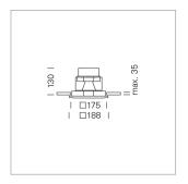
Recessed luminaire with LED, rated life of the LED L80/B10 > 50000 h, chromaticity tolerance 3 SDCM (initial), reflector with circular light distribution pattern, reflector pure aluminium 99,99% in MIRO-Silver®, swivel angle 30°, luminaire housing sheet steel, powder-coated, stratowhite, separate driver unit
