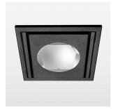
Recessed luminaire with LED, rated life of the LED L80/B10 > 50000 h, colour rendering index CRI > 80, chromaticity tolerance 3 SDCM (initial), reflector with oval light distribution pattern, reflector pure aluminium 99,99% in MIRO-Silver®, swivel angle 30°, luminaire housing sheet steel, powder-coated, stratoblack, separate driver unit
