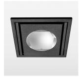
Recessed luminaire with LED, rated life of the LED L80/B10 > 50000 h, colour rendering index CRI > 90, chromaticity tolerance 2 SDCM (initial), reflector with oval light distribution pattern, reflector pure aluminium 99,99% in MIRO-Silver®, swivel angle 30°, luminaire housing sheet steel, powder-coated, stratoblack, separate driver unit
