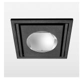
Recessed luminaire with LED, rated life of the LED L80/B10 > 50000 h, chromaticity tolerance 3 SDCM (initial), reflector with oval light distribution pattern, reflector pure aluminium 99,99% in MIRO-Silver®, swivel angle 30°, luminaire housing sheet steel, powder-coated, stratoblack, separate driver unit
