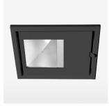
Recessed luminaire with LED, rated life of the LED L80/B10 > 50000 h, chromaticity tolerance 3 SDCM (initial), reflector with asymmetrical light distribution pattern, reflector pure aluminium 99,99% in MIRO-Silver®, swivel angle 30°, luminaire housing sheet steel, powder-coated, stratoblack, separate driver unit
