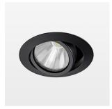
Recessed luminaire with LED, rated life of the LED L80/B10 > 50000 h, colour rendering index CRI > 90, chromaticity tolerance 3 SDCM (initial), rotation-symmetrical reflector with circular light distribution pattern, reflector pure aluminium 99,99% in MIRO-Silver®, segmented and faceted, 3D lens silicon to reduce the proportion of scattered light, die-cast aluminium, powder-coated, rotation angle, swivel angle +25° / -25°, stratoblack,
