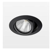
Recessed luminaire with LED, rated life of the LED L80/B10 > 50000 h, colour rendering index CRI > 80, chromaticity tolerance 3 SDCM (initial), rotation-symmetrical reflector with circular light distribution pattern, reflector pure aluminium 99,99% in MIRO-Silver®, segmented and faceted, 3D lens silicon to reduce the proportion of scattered light, die-cast aluminium, powder-coated, rotation angle , swivel angle +25° / -25°, stratoblack,
