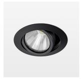
Recessed luminaire with LED, rated life of the LED L80/B10 > 50000 h, colour rendering index CRI > 80, chromaticity tolerance 3 SDCM (initial), rotation-symmetrical reflector with circular light distribution pattern, reflector pure aluminium 99,99% in MIRO-Silver®, segmented and faceted, 3D lens silicon to reduce the proportion of scattered light, die-cast aluminium, powder-coated, rotation angle, swivel angle +25°/-25°, stratoblack,
