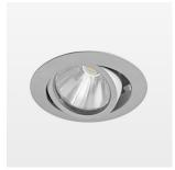
Recessed luminaire with LED, rated life of the LED L80/B10 > 50000 h, colour rendering index CRI > 90, chromaticity tolerance 3 SDCM (initial), rotation-symmetrical reflector with circular light distribution pattern, reflector pure aluminium 99,99% in MIRO-Silver®, segmented and faceted, 3D lens silicon to reduce the proportion of scattered light, die-cast aluminium, powder-coated, rotation angle , swivel angle +25° / -25°, stratosilver,
