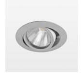
Recessed luminaire with LED, rated life of the LED L80/B10 > 50000 h, colour rendering index CRI > 80, chromaticity tolerance 3 SDCM (initial), rotation-symmetrical reflector with circular light distribution pattern, reflector pure aluminium 99,99% in MIRO-Silver®, segmented and faceted, 3D lens silicon to reduce the proportion of scattered light, die-cast aluminium, powder-coated, rotation angle , swivel angle +25° / -25°, stratosilver,
