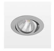
Recessed luminaire with LED, rated life of the LED L80/B10 > 50000 h, colour rendering index CRI > 90, chromaticity tolerance 2 SDCM (initial), rotation-symmetrical reflector with circular light distribution pattern, reflector pure aluminium 99,99% in MIRO-Silver®, segmented and faceted, 3D lens silicon to reduce the proportion of scattered light, die-cast aluminium, powder-coated, rotation angle , swivel angle +25° / -25°, stratosilver,
