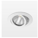
Recessed luminaire with LED, rated life of the LED L80/B10 > 50000 h, colour rendering index CRI > 90, chromaticity tolerance 3 SDCM (initial), rotation-symmetrical reflector with circular light distribution pattern, reflector pure aluminium 99,99% in MIRO-Silver®, segmented and faceted, 3D lens silicon to reduce the proportion of scattered light, die-cast aluminium, powder-coated, rotation angle , swivel angle  $\pm 25^{\circ}$  /  $\pm 25^{\circ}$ , stratowhite,
