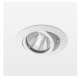
Recessed luminaire with LED, rated life of the LED L80/B10 > 50000 h, colour rendering index CRI > 80, chromaticity tolerance 3 SDCM (initial), rotation-symmetrical reflector with circular light distribution pattern, reflector pure aluminium 99,99% in MIRO-Silver®, segmented and faceted, 3D lens silicon to reduce the proportion of scattered light, die-cast aluminium, powder-coated, rotation angle , swivel angle  $\pm 25^{\circ}$  /  $\pm 25^{\circ}$ , stratowhite,
