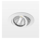
Recessed luminaire with LED, rated life of the LED L80/B10 > 50000 h, colour rendering index CRI > 90, chromaticity tolerance 2 SDCM (initial), rotation-symmetrical reflector with circular light distribution pattern, reflector pure aluminium 99,99% in MIRO-Silver®, segmented and faceted, 3D lens silicon to reduce the proportion of scattered light, die-cast aluminium, powder-coated, rotation angle , swivel angle  $\pm 25^{\circ}$  /  $\pm 25^{\circ}$ , stratowhite,
