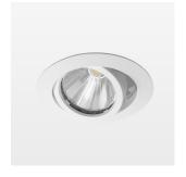
Recessed luminaire with LED, rated life of the LED L80/B10 > 50000 h, colour rendering index CRI > 95, chromaticity tolerance 2 SDCM (initial), rotation-symmetrical reflector with circular light distribution pattern, reflector pure aluminium 99,99% in MIRO-Silver®, segmented and faceted, 3D lens silicon to reduce the proportion of scattered light, die-cast aluminium, powder-coated, rotation angle , swivel angle +25° / -25°, stratowhite,
