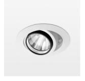
Recessed luminaire with LED, rated life of the LED L80/B10 > 50000 h, colour rendering index CRI > 96, chromaticity tolerance 2 SDCM (initial), rotation-symmetrical reflector with circular light distribution pattern, reflector pure aluminium 99,99% in MIRO-Silver®, segmented and faceted, 3D lens silicon to reduce the proportion of scattered light, die-cast aluminium, powder-coated, rotation angle , swivel angle  $+25^{\circ}/-25^{\circ}$ , stratowhite,
