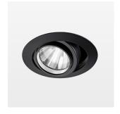
Recessed luminaire with LED, rated life of the LED L80/B10 > 50000 h, colour rendering index CRI > 90, chromaticity tolerance 2 SDCM (initial), rotation-symmetrical reflector with circular light distribution pattern, reflector pure aluminium 99,99% in MIRO-Silver®, segmented and faceted, 3D lens silicon to reduce the proportion of scattered light, die-cast aluminium, powder-coated, rotation angle , swivel angle  $\pm 25^{\circ}/ -25^{\circ}$ , stratoblack,
