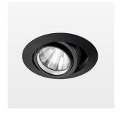
Recessed luminaire with LED, rated life of the LED L80/B10 > 50000 h, colour rendering index CRI > 96, chromaticity tolerance 2 SDCM (initial), rotation-symmetrical reflector with circular light distribution pattern, reflector pure aluminium 99,99% in MIRO-Silver®, segmented and faceted, 3D lens silicon to reduce the proportion of scattered light, die-cast aluminium, powder-coated, rotation angle , swivel angle  $\pm 25^{\circ}/ -25^{\circ}$ , stratoblack,
