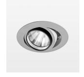
Recessed luminaire with LED, rated life of the LED L80/B10 > 50000 h, colour rendering index CRI > 96, chromaticity tolerance 2 SDCM (initial), rotation-symmetrical reflector with circular light distribution pattern, reflector pure aluminium 99,99% in MIRO-Silver®, segmented and faceted, 3D lens silicon to reduce the proportion of scattered light, die-cast aluminium, powder-coated, rotation angle , swivel angle  $\pm 25^{\circ}/ -25^{\circ}$ , stratosilver,
