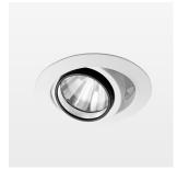
Recessed luminaire with LED, rated life of the LED L80/B10 > 50000 h, colour rendering index CRI > 90, chromaticity tolerance 2 SDCM (initial), rotation-symmetrical reflector with circular light distribution pattern, reflector pure aluminium 99,99% in MIRO-Silver®, segmented and faceted, 3D lens silicon to reduce the proportion of scattered light, die-cast aluminium, powder-coated, rotation angle, swivel angle +25°/-25°, stratowhite,
