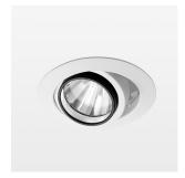
Recessed luminaire with LED, rated life of the LED L80/B10 > 50000 h, colour rendering index CRI > 80, chromaticity tolerance 2 SDCM (initial), rotation-symmetrical reflector with circular light distribution pattern, reflector pure aluminium 99,99% in MIRO-Silver®, segmented and faceted, 3D lens silicon to reduce the proportion of scattered light, die-cast aluminium, powder-coated, rotation angle , swivel angle +25°/ -25°, stratowhite,
