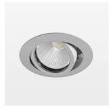
Recessed luminaire with LED, rated life of the LED L80/B10 > 50000 h, colour rendering index CRI > 80, chromaticity tolerance 2 SDCM (initial), reflector with circular light distribution pattern, reflector pure aluminium 99,99% in MIRO-Silver®, segmented and faceted, 3D lens silicon to reduce the proportion of scattered light, die-cast aluminium, powder-coated, rotation angle , swivel angle  $\pm 25^{\circ}$  /  $\pm 25^{\circ}$ , stratosilver,
