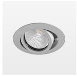
Recessed luminaire with LED, rated life of the LED L80/B10 > 50000 h, colour rendering index CRI > 96, chromaticity tolerance 2 SDCM (initial), reflector with circular light distribution pattern, reflector pure aluminium 99,99% in MIRO-Silver®, segmented and faceted, 3D lens silicon to reduce the proportion of scattered light, die-cast aluminium, powder-coated, rotation angle , swivel angle  $\pm 25^{\circ}$  /  $\pm 25^{\circ}$ , stratosilver,
