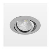
Recessed luminaire with LED, rated life of the LED L80/B10 > 50000 h, colour rendering index CRI > 96, chromaticity tolerance 2 SDCM (initial), reflector with circular light distribution pattern, reflector pure aluminium 99,99% in MIRO-Silver®, segmented and faceted, 3D lens silicon to reduce the proportion of scattered light, die-cast aluminium, powder-coated, rotation angle , swivel angle +25° / -25°, stratosilver,
