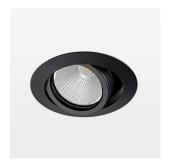
Recessed luminaire with LED, rated life of the LED L80/B10 > 50000 h, colour rendering index CRI > 80, chromaticity tolerance 2 SDCM (initial), reflector with circular light distribution pattern, reflector pure aluminium 99,99% in MIRO-Silver®, segmented and faceted, 3D lens silicon to reduce the proportion of scattered light, die-cast aluminium, powder-coated, rotation angle , swivel angle +25° / -25°, stratoblack,
