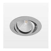
Recessed luminaire with LED, rated life of the LED L80/B10 > 50000 h, colour rendering index CRI > 90, chromaticity tolerance 2 SDCM (initial), reflector with circular light distribution pattern, reflector pure aluminium 99,99% in MIRO-Silver®, segmented and faceted, 3D lens silicon to reduce the proportion of scattered light, die-cast aluminium, powder-coated, rotation angle , swivel angle +25° / -25°, stratosilver,
