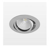
Recessed luminaire with LED, rated life of the LED L80/B10 > 50000 h, colour rendering index CRI > 80, chromaticity tolerance 2 SDCM (initial), reflector with circular light distribution pattern, reflector pure aluminium 99,99% in MIRO-Silver®, segmented and faceted, 3D lens silicon to reduce the proportion of scattered light, die-cast aluminium, powder-coated, rotation angle , swivel angle +25° / -25°, stratosilver,
