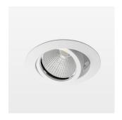
Recessed luminaire with LED, rated life of the LED L80/B10 > 50000 h, colour rendering index CRI > 90, chromaticity tolerance 2 SDCM (initial), reflector with circular light distribution pattern, reflector pure aluminium 99,99% in MIRO-Silver®, segmented and faceted, 3D lens silicon to reduce the proportion of scattered light, die-cast aluminium, powder-coated, rotation angle , swivel angle +25° / -25°, stratowhite,
