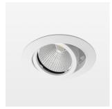
Recessed luminaire with LED, rated life of the LED L80/B10 > 50000 h, colour rendering index CRI > 80, chromaticity tolerance 2 SDCM (initial), reflector with circular light distribution pattern, reflector pure aluminium 99,99% in MIRO-Silver®, segmented and faceted, 3D lens silicon to reduce the proportion of scattered light, die-cast aluminium, powder-coated, rotation angle , swivel angle  $\pm 25^{\circ}$  /  $\pm 25^{\circ}$ , stratowhite,
