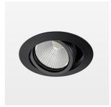
Recessed luminaire with LED, rated life of the LED L80/B10 > 50000 h, colour rendering index CRI > 80, chromaticity tolerance 2 SDCM (initial), reflector with circular light distribution pattern, reflector pure aluminium 99,99% in MIRO-Silver®, segmented and faceted, die-cast aluminium, powder-coated, rotation angle , swivel angle +25° / -25°, stratoblack,
