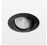
Recessed luminaire with LED, rated life of the LED L80/B10 > 50000 h, colour rendering index CRI > 90, chromaticity tolerance 2 SDCM (initial), reflector with circular light distribution pattern, reflector pure aluminium 99,99% in MIRO-Silver®, segmented and faceted, die-cast aluminium, powder-coated, rotation angle , swivel angle +25° / -25°, stratosilver,
