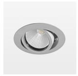
Recessed luminaire with LED, rated life of the LED L80/B10 > 50000 h, colour rendering index CRI > 80, chromaticity tolerance 2 SDCM (initial), reflector with circular light distribution pattern, reflector pure aluminium 99,99% in MIRO-Silver®, segmented and faceted, die-cast aluminium, powder-coated, rotation angle , swivel angle +25° / -25°, stratosilver,
