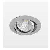
Recessed luminaire with LED, rated life of the LED L80/B10 > 50000 h, colour rendering index CRI > 80, chromaticity tolerance 2 SDCM (initial), reflector with circular light distribution pattern, reflector pure aluminium 99,99% in MIRO-Silver®, segmented and faceted, die-cast aluminium, powder-coated, rotation angle , swivel angle +25° / -25°, stratosilver,
