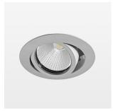
Recessed luminaire with LED, rated life of the LED L80/B10 > 50000 h, colour rendering index CRI > 90, chromaticity tolerance 2 SDCM (initial), reflector with circular light distribution pattern, reflector pure aluminium 99,99% in MIRO-Silver®, segmented and faceted, die-cast aluminium, powder-coated, rotation angle , swivel angle +25° / -25°, stratosilver,
