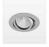
Recessed luminaire with LED, rated life of the LED L80/B10 > 50000 h, colour rendering index CRI > 96, chromaticity tolerance 2 SDCM (initial), reflector with circular light distribution pattern, reflector pure aluminium 99,99% in MIRO-Silver®, segmented and faceted, die-cast aluminium, powder-coated, rotation angle , swivel angle +25° / -25°, stratosilver,
