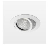
Recessed luminaire with LED, rated life of the LED L80/B10 > 50000 h, colour rendering index CRI > 90, chromaticity tolerance 2 SDCM (initial), reflector with circular light distribution pattern, reflector pure aluminium 99,99% in MIRO-Silver®, segmented and faceted, die-cast aluminium, powder-coated, rotation angle , swivel angle +25° / -25°, stratowhite,
