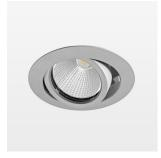
Recessed luminaire with LED, rated life of the LED L80/B10 > 50000 h, colour rendering index CRI > 96, chromaticity tolerance 2 SDCM (initial), reflector with circular light distribution pattern, reflector pure aluminium 99,99% in MIRO-Silver®, segmented and faceted, die-cast aluminium, powder-coated, rotation angle , swivel angle +25° / -25°, stratosilver,
