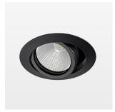
Recessed luminaire with LED, rated life of the LED L80/B10 > 50000 h, colour rendering index CRI > 90, chromaticity tolerance 2 SDCM (initial), reflector with circular light distribution pattern, reflector pure aluminium 99,99% in MIRO-Silver®, segmented and faceted, die-cast aluminium, powder-coated, rotation angle , swivel angle +25° / -25°, stratoblack,
