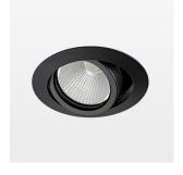
Recessed luminaire with LED, rated life of the LED L80/B10 > 50000 h, colour rendering index CRI > 96, chromaticity tolerance 2 SDCM (initial), reflector with circular light distribution pattern, reflector pure aluminium 99,99% in MIRO-Silver®, segmented and faceted, die-cast aluminium, powder-coated, rotation angle , swivel angle +25° / -25°, stratoblack,
