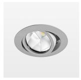
Recessed luminaire with LED, rated life of the LED L80/B10 > 50000 h, colour rendering index CRI > 96, chromaticity tolerance 2 SDCM (initial), reflector with oval light distribution pattern, reflector pure aluminium 99,99% in MIRO-Silver®, segmented, die-cast aluminium, powder-coated, rotation angle , swivel angle  $\pm 25^{\circ}$  /  $\pm 25^{\circ}$ , stratosilver,
