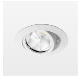
Recessed luminaire with LED, rated life of the LED L80/B10 > 50000 h, colour rendering index CRI > 96, chromaticity tolerance 2 SDCM (initial), reflector with oval light distribution pattern, reflector pure aluminium 99,99% in MIRO-Silver®, segmented, die-cast aluminium, powder-coated, rotation angle , swivel angle  $\pm 25^{\circ}$  /  $\pm 25^{\circ}$ , stratowhite,
