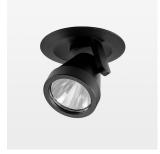
Semi-recessed luminaire with LED, rated life of the LED L80/B10 > 50000 h, colour rendering index CRI > 95, chromaticity tolerance 2 SDCM (initial), rotation-symmetrical reflector with circular light distribution pattern, reflector pure aluminium 99,99% in MIRO-Silver®, segmented and faceted, 3D lens silicon to reduce the proportion of scattered light, die-cast aluminium, powdercoated, rotation angle 400°, swivel angle +85° / -85°, stratoblack, separate driver unit
