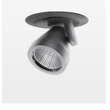
Semi-recessed luminaire with LED, rated life of the LED L80/B10 > 50000 h, colour rendering index CRI > 96, chromaticity tolerance 2 SDCM (initial), rotation-symmetrical reflector with circular light distribution pattern, reflector pure aluminium 99,99% in MIRO-Silver®, segmented and faceted, 3D lens silicon to reduce the proportion of scattered light, die-cast aluminium, powder-coated, rotation angle 400°, swivel angle +85° / -85°, stratosilver, separate driver unit
