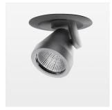
Semi-recessed luminaire with LED, rated life of the LED L80/B10 > 50000 h, colour rendering index CRI > 96, chromaticity tolerance 2 SDCM (initial), rotation-symmetrical reflector with circular light distribution pattern, reflector pure aluminium 99,99% in MIRO-Silver®, segmented and faceted, 3D lens silicon to reduce the proportion of scattered light, die-cast aluminium, powdercoated, rotation angle 400°, swivel angle +85°/-85°, stratosilver, separate driver unit
