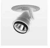
Semi-recessed luminaire with LED, rated life of the LED L80/B10 > 50000 h, colour rendering index CRI > 96, chromaticity tolerance 2 SDCM (initial), rotation-symmetrical reflector with circular light distribution pattern, reflector pure aluminium 99,99% in MIRO-Silver®, segmented and faceted, 3D lens silicon to reduce the proportion of scattered light, die-cast aluminium, powder-coated, rotation angle 400°, swivel angle +85° / -85°, stratowhite, separate driver unit
