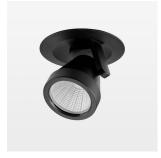
Semi-recessed luminaire with LED, rated life of the LED L80/B10 > 50000 h, colour rendering index CRI > 96, chromaticity tolerance 2 SDCM (initial), reflector with circular light distribution pattern, reflector pure aluminium 99,99% in MIRO-Silver®, segmented and faceted, 3D lens silicon to reduce the proportion of scattered light, die-cast aluminium, powder-coated, rotation angle 400°, swivel angle +85° / -85°, stratoblack, separate driver unit
