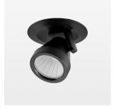
Semi-recessed luminaire with LED, rated life of the LED L80/B10 > 50000 h, colour rendering index CRI > 90, chromaticity tolerance 2 SDCM (initial), reflector with circular light distribution pattern, reflector pure aluminium 99,99% in MIRO-Silver®, segmented and faceted, 3D lens silicon to reduce the proportion of scattered light, die-cast aluminium, powder-coated, rotation angle 400°, swivel angle +85° / -85°, stratoblack, separate driver unit
