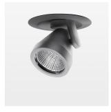
Semi-recessed luminaire with LED, rated life of the LED L80/B10 > 50000 h, colour rendering index CRI > 90, chromaticity tolerance 2 SDCM (initial), reflector with circular light distribution pattern, reflector pure aluminium 99,99% in MIRO-Silver®, segmented and faceted, 3D lens silicon to reduce the proportion of scattered light, die-cast aluminium, powder-coated, rotation angle 400°, swivel angle +85° / -85°, stratosilver, separate driver unit
