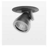
Semi-recessed luminaire with LED, rated life of the LED L80/B10 > 50000 h, colour rendering index CRI > 96, chromaticity tolerance 2 SDCM (initial), reflector with circular light distribution pattern, reflector pure aluminium 99,99% in MIRO-Silver®, segmented and faceted, 3D lens silicon to reduce the proportion of scattered light, die-cast aluminium, powder-coated, rotation angle 400°, swivel angle +85° / -85°, stratosilver, separate driver unit
